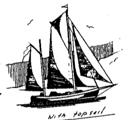
William Garden designed alternative rig and cabin house arrangements for the Bull Frog: shown is a ketch rig with a long coachroof. (Courtesy William Garden)
