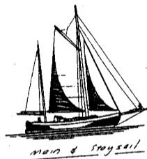
William Garden designed alternative rig and cabin house arrangements for the Bull Frog: shown is a ketch rig with a long coachroof. (Courtesy William Garden)
